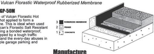
Materials are heated on site using a mechanically agitated oil heated Asphalt Mixer machine. The reheating and control of materials shall be carried out by an operator who has been factory trained and shall be thoroughly skilled in the operation of the machinery and have complete knowledge of the use and application of salt resistant rubberized thermoplastic coatings and a comprehensive knowledge of all materials used in the manufacturing.
